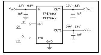
Figure 22. Typical Application Circuit
